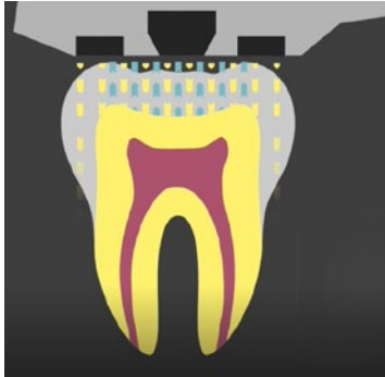
The iTero Element 5D intraoral scanner uses light of 850nm that penetrates into the tooth structure to produce a NIRI image.
