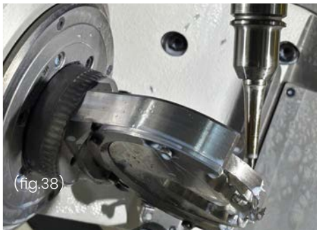
Examples of machining with a heat-shrink spindle
