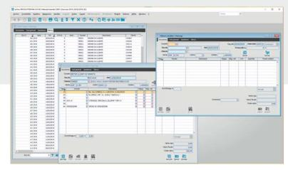
MillBox receives a production order from the management system, then creates a new project (for example with the name of the order), loads the objects according to their type to the machine that will perform the machinings and the material to be used, also taking into account its possible color.
