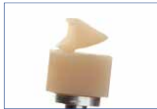
Crown directly after milling
