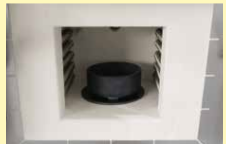
Loading in the sintering furnace LT 02/13 CR
