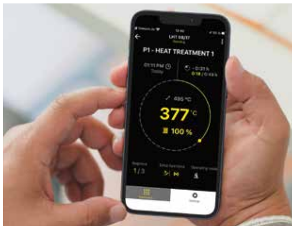
Display of program progress for each furnace
