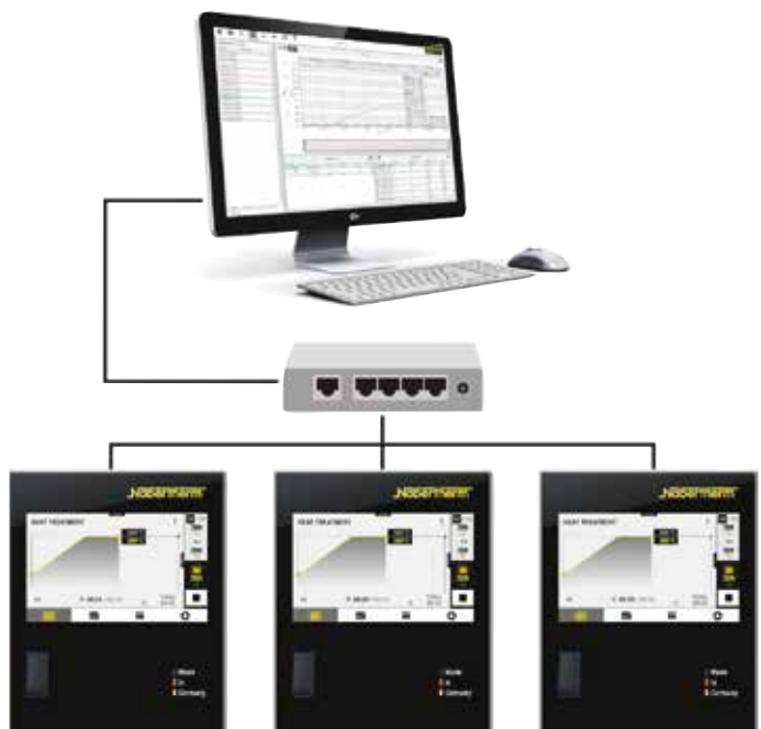
Example lay-out with 3 furnaces
