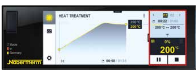
Detailed overview of process information including setpoint, actual value and switched functions
